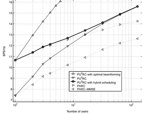
Figure 5: Throughput performance of PU<sup>2</sup>RC with hybrid scheduling over other schemes
