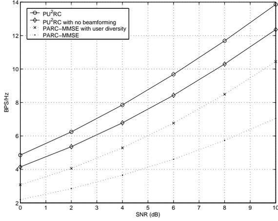
Figure 3: Throughput comparison of PU<sup>2</sup>RC and PARC-MMSE
