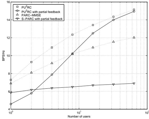
Figure 4: Throughput comparison of PU<sup>2</sup>RC, PARC-MMSE, and S-PARC
