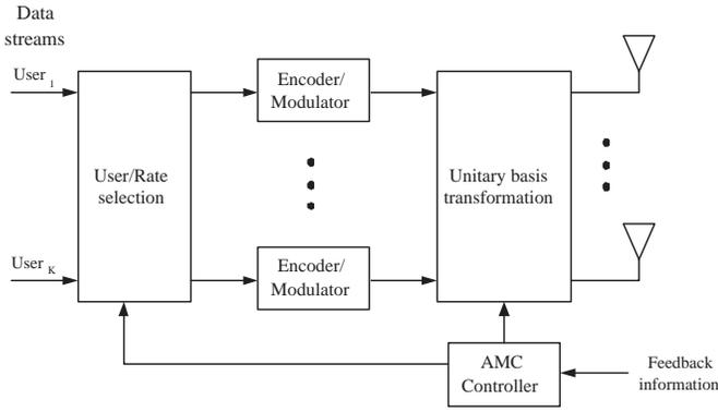
Figure 2: Schematic of PU<sup>2</sup>RC transmitter
